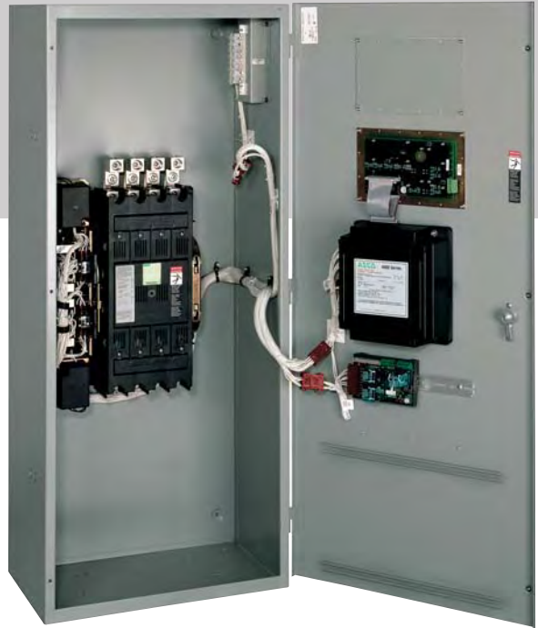
Fig. 3: Four pole, Delayed-Transition Transfer Switch rated 400 amperes in Type 1 enclosure.
